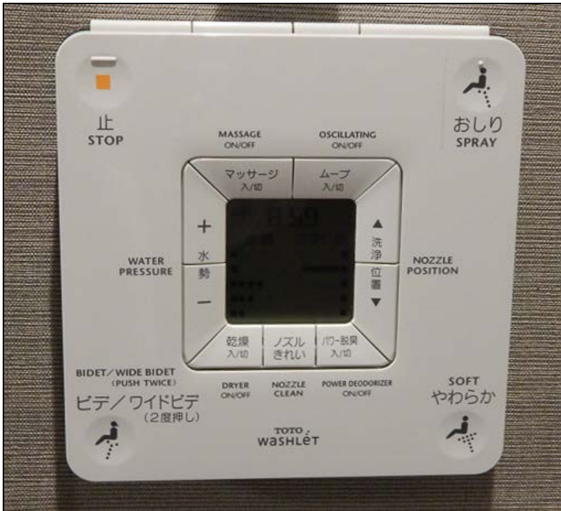
Control panel for Japanese toilet.
